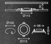
PROFONDEUR D'INSTALLATION | MOUNTING DEPTH | EINBAUTIEFE 40MM
